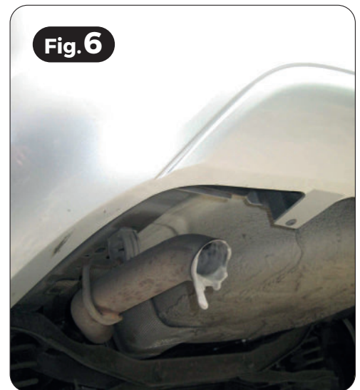
J02256 | JLM Diesel DPF Probe Spray gun with probe for direct spraying on monolith
